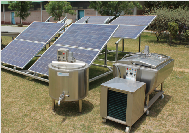
Figure 1. Actual view of energy efficient solar based milk chiller unit
